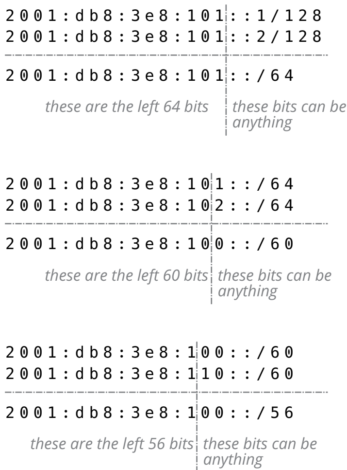
Figure 5-7 Aggregation and Reachable Destinations in IPv6 Addressing
