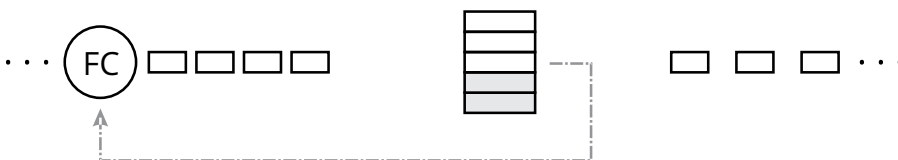
Figure 2-10 A Feedback Loop to Control Packet Flow
